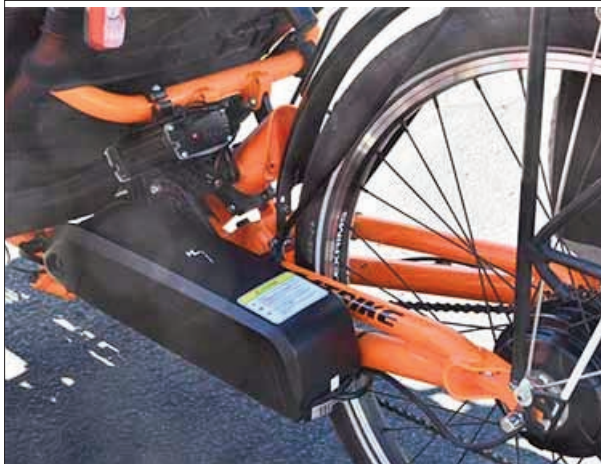
The Encased Battery
